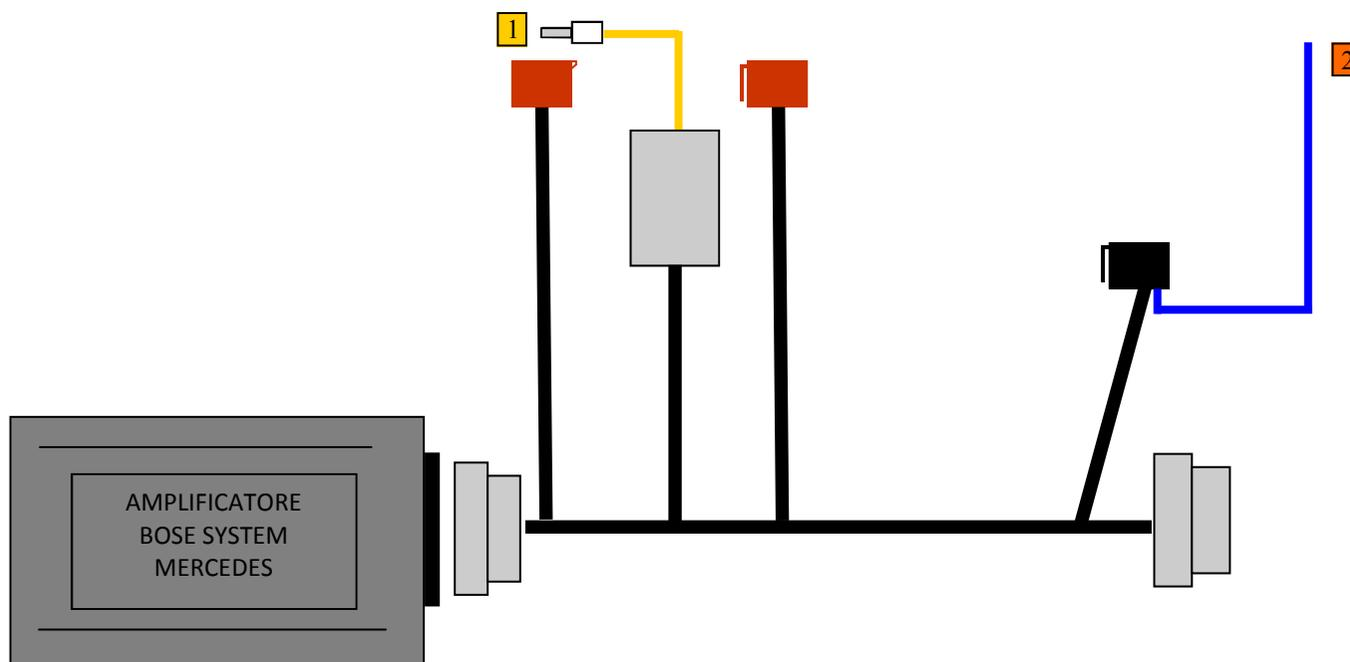
CONNESSIONI CON CABLAGGIO **CP143** PER SISTEMI BOSE
