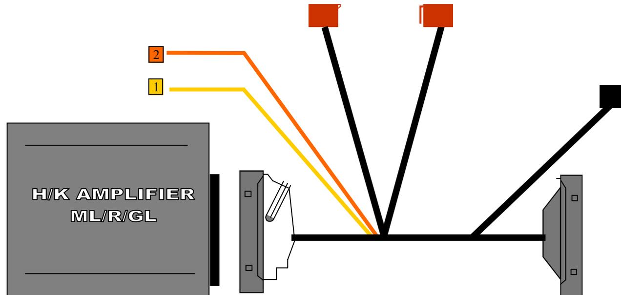
CONNESSIONI CON CABLAGGIO **CP149** PER SISTEMI HARMAN KARDON
