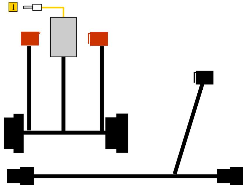
CONNESSIONI CON CABLAGGIO CP148 PER SISTEMI HARMAN KARDON 9 ALTOPARLANTI
